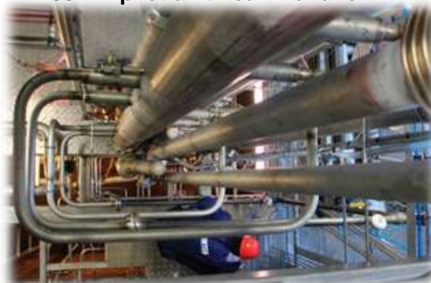
Chemical Looping Combustion 150 kW pilot unit near Trondheim:
